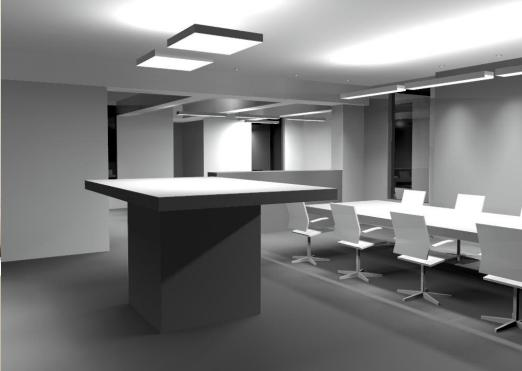
A well balanced illuminated environment was essential, providing illumination on to the high ceilings and also the verticals within the space. The design was developed in line with BS EN 12464-1 office standards, with lighting purely focused on the task areas within the space. The scheme provided an efficient lighting design with a delivery of light which followed the functions and tasks within each office area.
